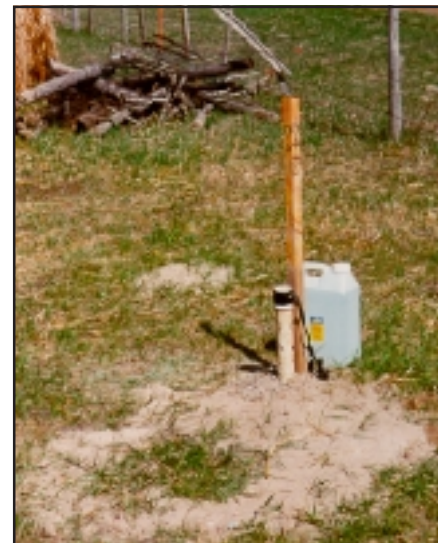
A monitoring well
