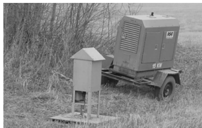
VIDO Air Sampler - upwind location
